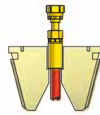
GF FITTING SWIVEL Compression Cross-Section View
